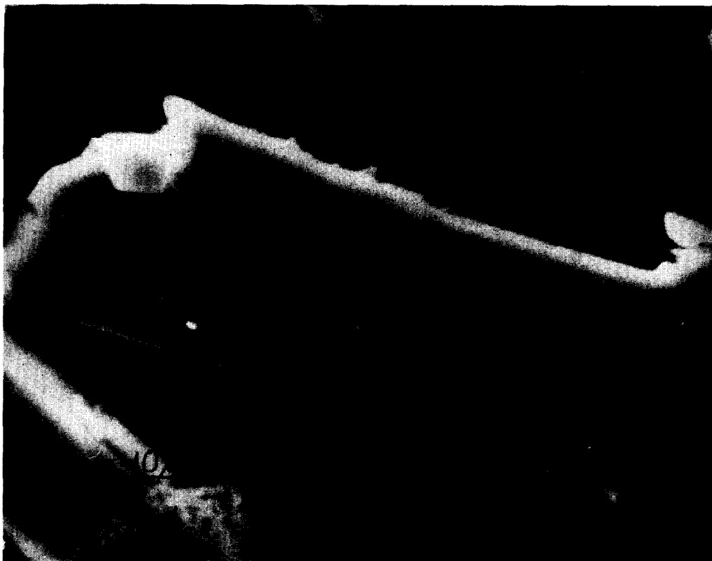
FIG. 1. Electron probe microanalysis of V_2O_5 catalyst containing 10 mole% MoO_3 . (a) Electron image of the sample (Compo). 1, 2, and 3 signify spots chosen for the quantitative X-ray microanalysis; (b) Mo analysis of the same area in a fresh catalyst; (c) the same as (b) but after a cycle of oxidizing and reducing treatments.
